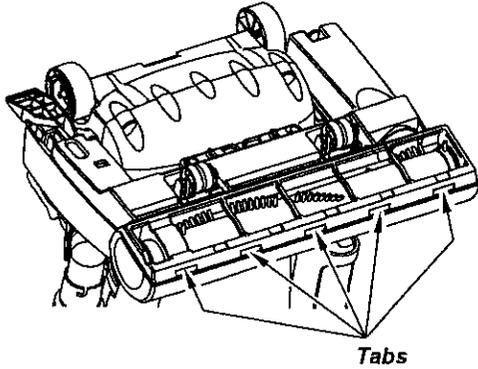
As the base is lowered the inner areas will brush against the dust compartment wheels.
